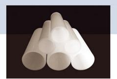
QT402 In flexible two step process (QT402), very pure quartz sand is electrically fused to form quartz glass ingot. Then remelt the ingot by the furnace, drawing the tube. The range of drawn tubes covers an outer diameter of 8-120mm with a wall thickness depending on the outer diameter.
